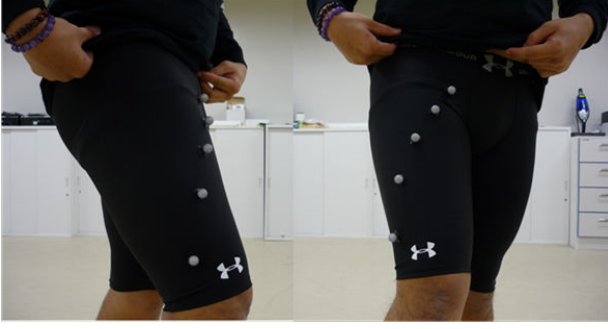
Figure 10. Arrangement of markers for motion capture
