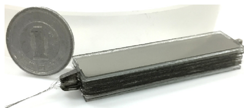
Fig. 5. A sample of fabricated 10-layer multilayered PVC gel artificial muscles with a one-yen coin.
